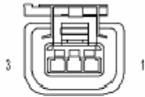
SENSOR- CAMSHAFT POSITION (DIESEL)
