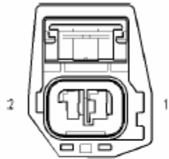
SENSOR- WHEEL SPEED-ABS- LEFT REAR (ESP)
