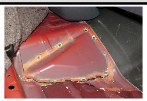
5. Remove the fasteners and sealer from around the patch panel. Cut away the sound deadener pad to expose the transmission PTO access.
