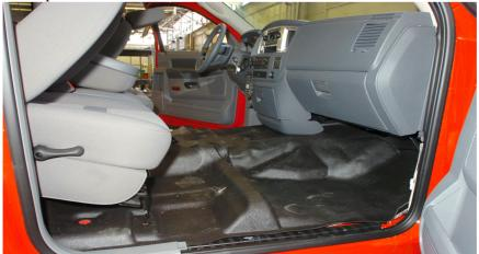
4. Lift the floor mat and fold it rearward and toward the drivers side to expose the patch panel
