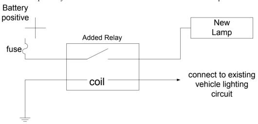
When this type of circuit is used please understand that there is no way for the vehicle to perform any diagnostics on the added lamps.
