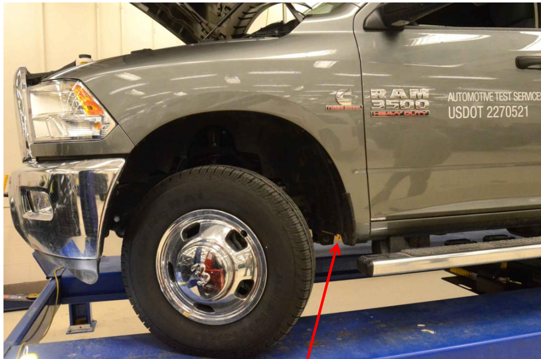
Connector located behind the left (driver's side) front wheel well liner
