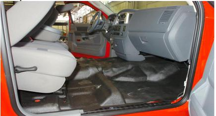
4. Lift the floor mat and fold it rearward and toward the drivers side to expose the patch panel
