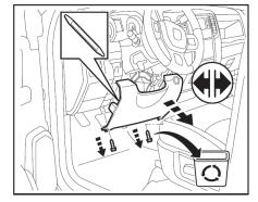
2.- Locate the two gray connectors: one 4 way connector (on the right side near the plastic panel where the knee blocker attached) and one 2 way connector (at the top of the gas pedal).
