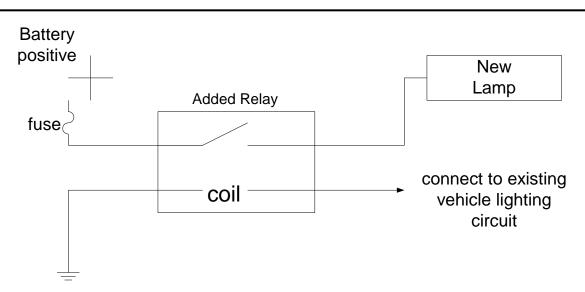
When this type of circuit is used please understand that there is no way for the vehicle to perform any diagnostics on the added lamps.
