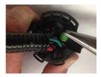
Insert the wire with terminal into the back of the connector, when fully seated, you should not be able to pull the terminal back out
