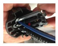
Remove the green rubber plug from the back of the connector
