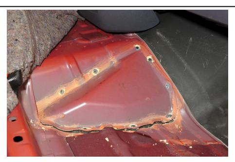
5. Remove the fasteners and sealer from around the patch panel. Cut away the sound deadener pad to expose the transmission PTO access.
