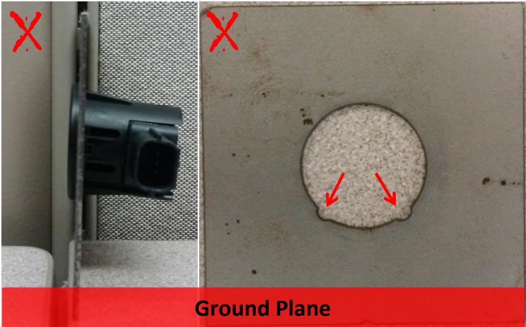
Figure 6: Incorrect coupon and Sensor Mounting
