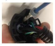
Re-install the lock and re-attach the harness connecter to the trailer connector
