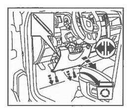
2. Locate the gray 4 way connector (on the right side near the plastic panel where the knee blocker attached).
