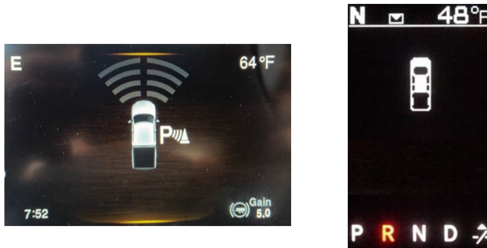
Figure 9: Instrument Cluster Graphic For With Only Front Sensors Installed (Highline Cluster Left – Midline Cluster Right)
