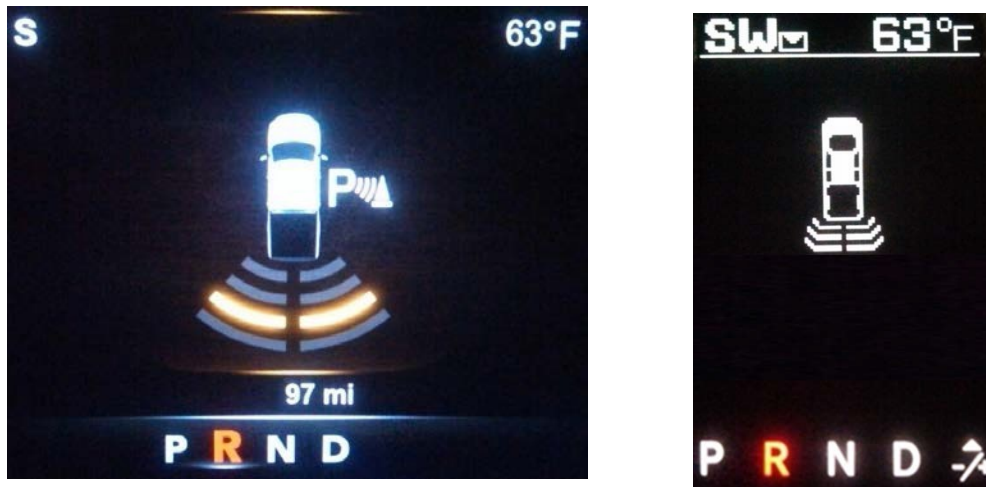
Figure 14: Cluster Graphic with object detected (Highline Cluster Left – Midline Cluster Right)
