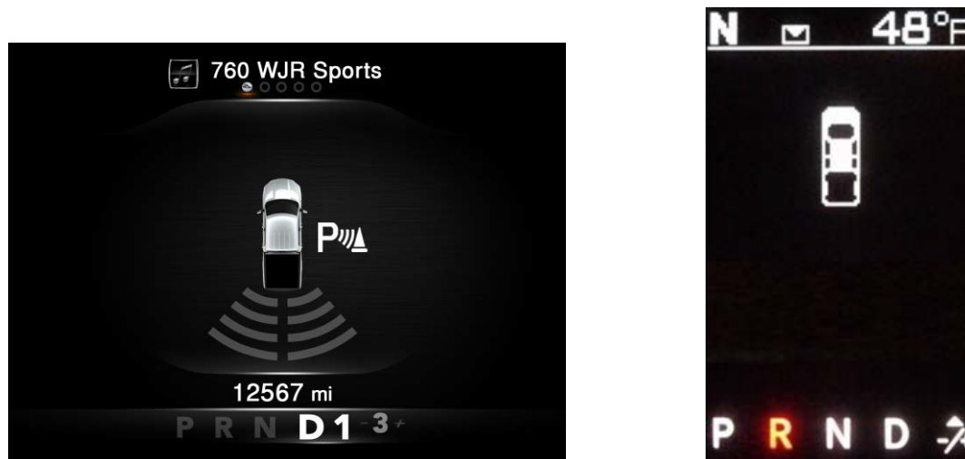
Figure 13: Instrument Cluster Graphic with no obstructions detected (Highline Cluster Left – Midline Cluster Right)
