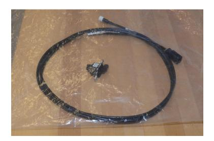
To install, first remove the video cable and the camera from the upfitter bag, extend the cable to locate both end-connectors. Install the *white* connector from jumper onto the camera connector mate as shown in the pictures. A 'click' will be heard when a secure connection has been achieved.
